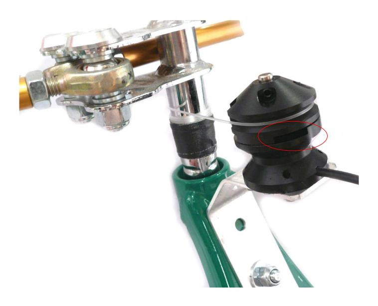
3) Turn the steering wheel from the LEFT to the RIGHT and vice-versa to check the good working of the potentiometer. The string must not overlap its self.
