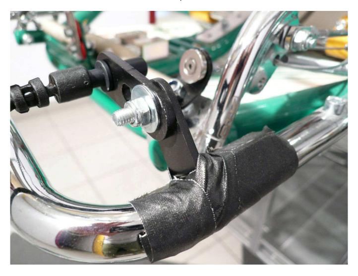
On this second example, we applied a high quality adhesive tape to fix the support of the sensor.
