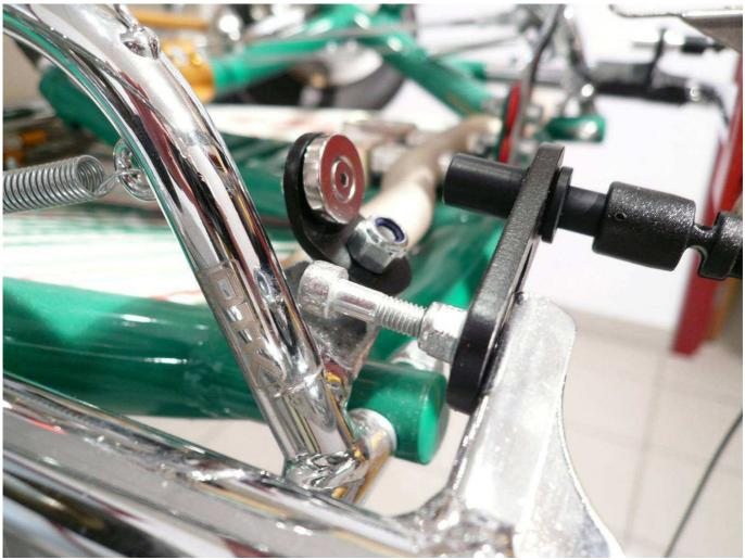
**Warning**: if you bend the magnetic support (like on the image) so that it's +/- facing the sensor, please first remove the magnet.
